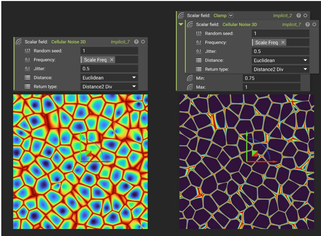
We want to etch this field into the part, so we use a negative value in the Multiply block. This offsets the creases (high spots in the field) inwards.
