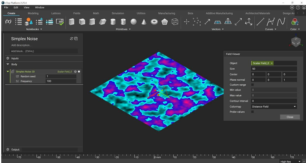
Using the field viewer (press F), you can see that the noise ranges from -1 to 1 (toggle “Probe Values” on the Field Viewer dialog, and hover over the field). The influence of the frequency input is best visualized by changing the value, and the random seed is useful if you want to layer multiple noise functions without them coinciding, or to randomize different parts’ textures.
