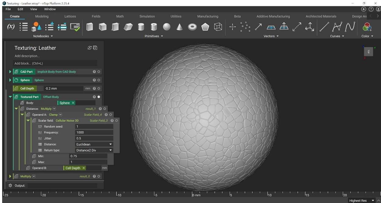
In between our Noise and Multiply block, we use a Clamp. This essentially thresholds the noise signal (which runs from 0 to 1) to be between 0.75 and 1 only. This will create flat spots in our leather cells, rather than mountains, and is easier to visualize with the Turbo option in the Field Viewer.
