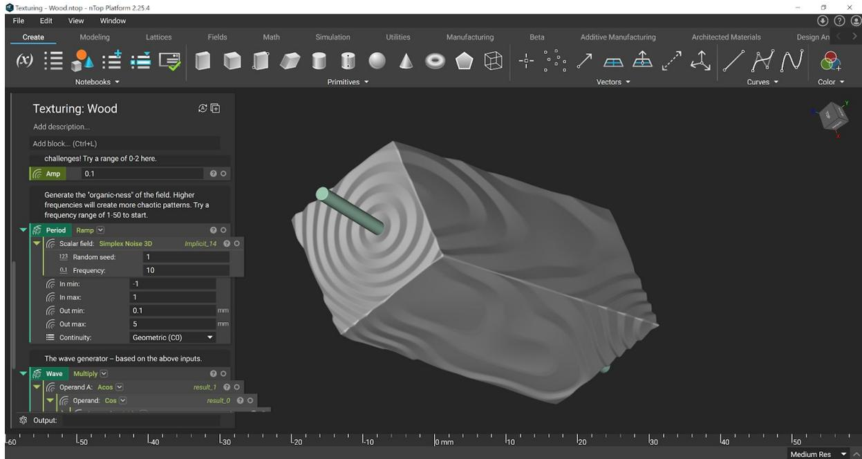
The period of the waves can be linked to noise functions, allowing control over how chaotic the rings look. With a high frequency value, the texture may begin to resemble some sort of magnetic material instead.
