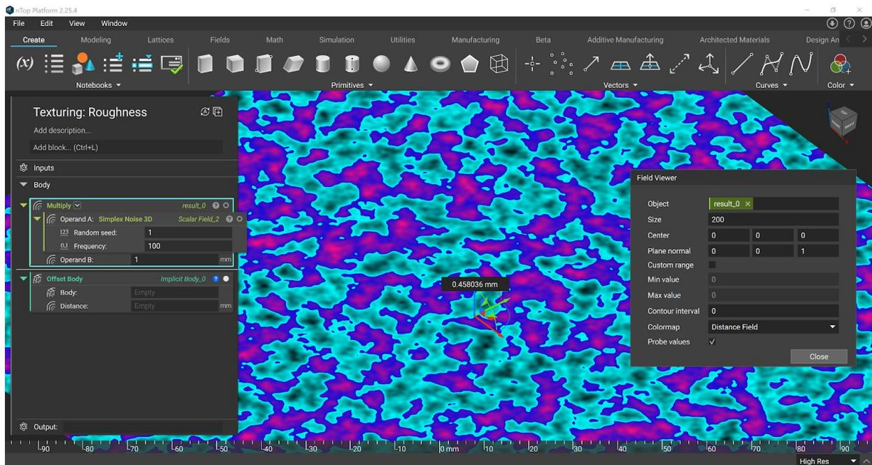
The resulting field now has units of length, and can be used in an Offset block to add and remove material (the original sphere is shown in green). The magnitude of this multiplying value controls the depth or strength of the texture, and can be varied spatially (as indicated by the curved field icon
