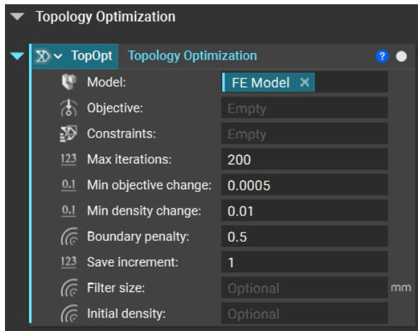
**Step 2:** The Objective input is where we define what we want to gain out of this Topology Optimization. Often, we'll assign multiple design responses to give various load cases. This is more realistic, as most parts aren't subjected to only one load case.
