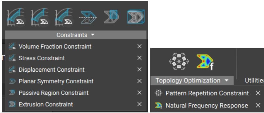
For this example, apply a **Volume Fraction Constraint** and a **Planar Symmetry Constraint** in the Constraints list of the Topology Optimization block.
