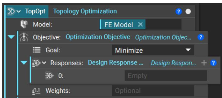
When applying multiple Objectives, we can use the Weights input to assign different weightings to each Objective. If the Weights input is left blank, all Objectives will be given the same weighting.
