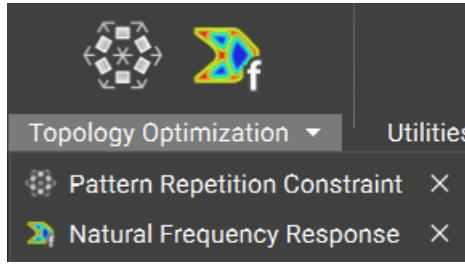
Add a **Structural Compliance Response** to the Notebook. Pull this into the Design Response input in the Objective block. For the Goal, select Minimize from the drop-down menu because we aim for minimal deformation in this part. For the Load case, assign the two Boundary Conditions established in the last lesson.
