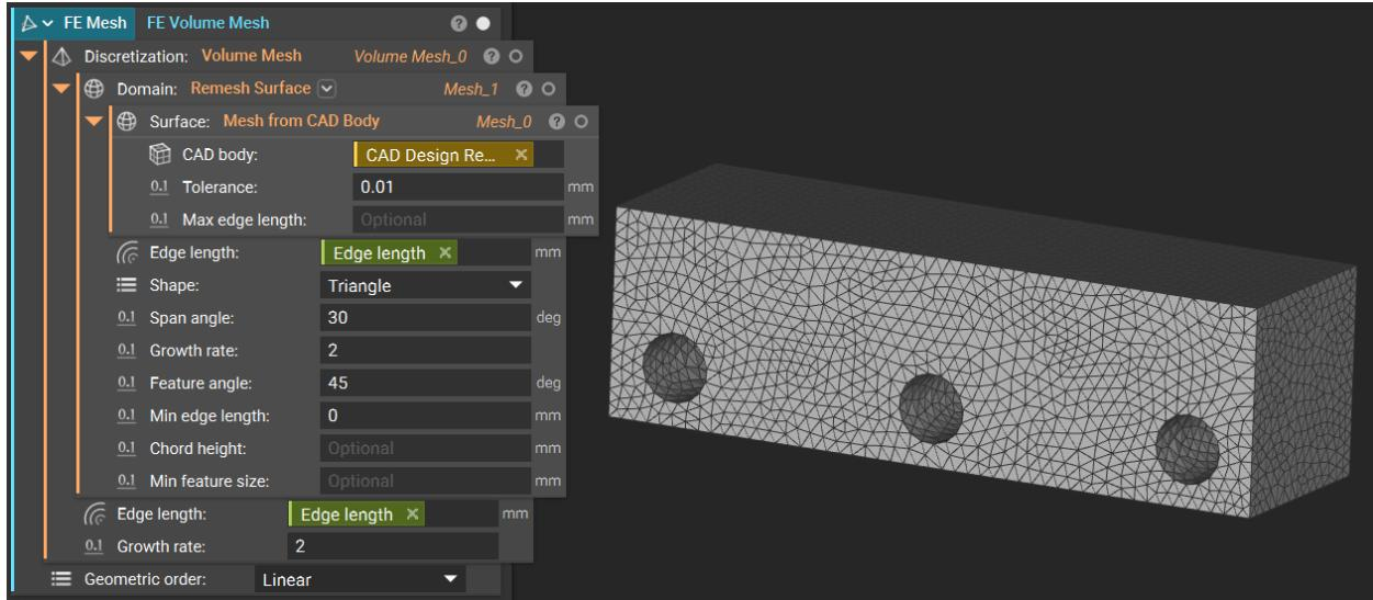
**Step 5:** Now, we'll use our FE Mesh as a component in an FE Model. Add an **FE Model** block to your Notebook. In the Components List, add an **FE Component** block. Use the *FE Mesh* variable as the Mesh input.
