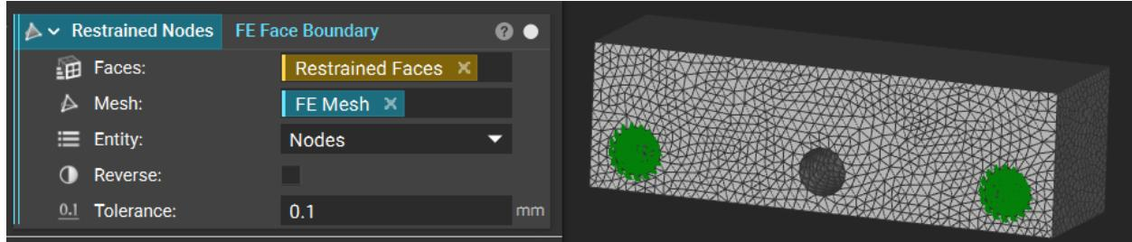
Once these nodes are selected, add a **Displacement Restraint** block to the Notebook. Use the *Restrained Nodes* as your input, and leave all other inputs as 0. This indicates zero translation or rotation of all selected nodes. Make this block a variable called *Fixed Restraint*. You've now created your first of two boundary conditions.
