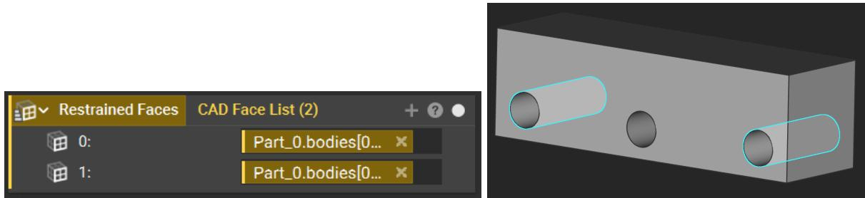
Then, select the middle hole, select “Create CAD Face Variable” (since this is a single face and not a list), and rename this variable *Loaded Face*.
