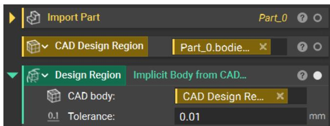
**Step 2:** Holding CTRL on your keyboard, click on each of the three holes in the CAD Design Region, then right-click and choose “Create CAD Face List Variable” from the dropdown menu. Rename this variable *Interfaces*. These holes will be the interfaces at which we set our boundary conditions later in the workflow—the two outer holes will be restrained, and a load will be applied to the middle hole via a force vector.
