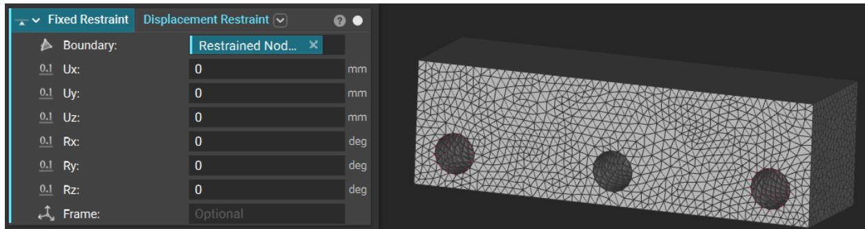
**Step 7:** Finally, let's establish the boundary condition at the loaded hole. To select the center hole, we could use the **FE Face Boundary** block we used in Step 6, but let's explore another option for selecting our nodes.
