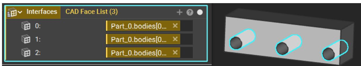
**Step 3:** Now, we'll specify the CAD faces which will be restrained and that which will be loaded. Using the same process as in Step 2, select the two outer holes and create a variable named *Restrained Faces*.
