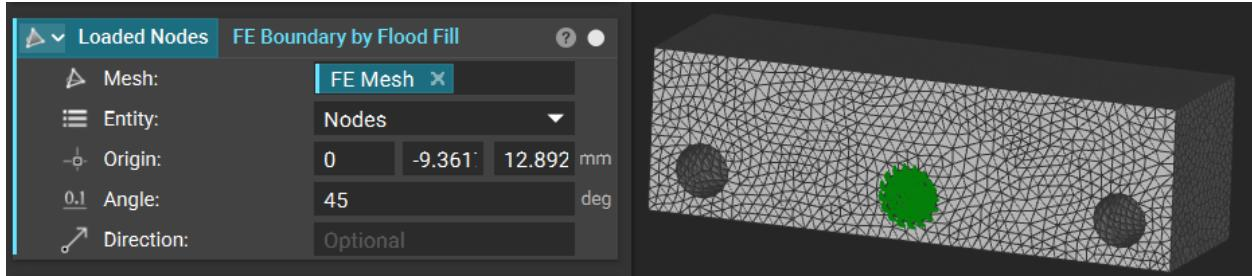
Finally, to apply a load to this feature, add a **Force** block to the Notebook. Use *Loaded Nodes* as the Boundary and input a vector of [0,-1000,0] N, indicating a force of 1000 Newtons in the negative y-direction. This load will be distributed among all the nodes in our *Loaded Nodes* boundary. Make this into a variable called **Force**. You've now successfully created your second boundary condition.
