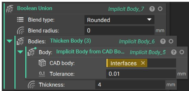
We'll add another Boolean Union block to merge these three holes with our Smooth Body variable to make a single part with our interfaces and Top-opt results. To smooth the blend, set the Blend radius to 1mm.
