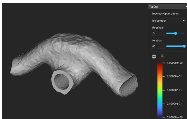
The Iso-contour option shows this single surface with elements meeting the nominal Threshold, which can be modified using this slider. When the Threshold equals 0, our initial part can be seen, and as it moves toward 1, we see the gradual removal of elements with lower top-opt densities. The iterations slider shows the evolution of the top-opt through each iteration.
