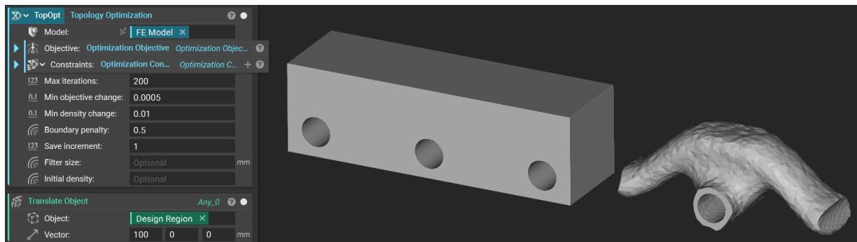
**Step 3:** Since Topology Optimization works by assigning a density value between 0 and 1 to each mesh element, we can use the Topology Optimization window to better understand how the calculated densities have affected our part and how the output meets our objective.
