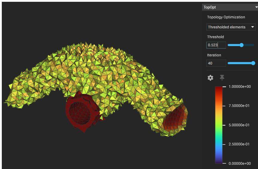
**Step 5:** Opening up the settings in our results window, we can control the color palette of our elements, whether the gradient is continuous or banded, and the preferred number of color bands.
