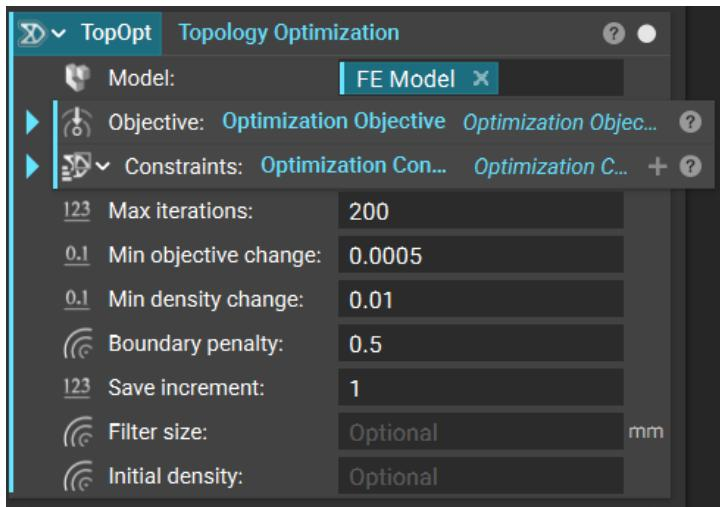
The input for Max iterations is pre-populated with a value of 200. Because Topology Optimization is iterative, we can set a limit for the number of iterations attempted. For more complex optimizations that may take longer to run, this should help users to reduce computation time with the slight tradeoff of accuracy.
