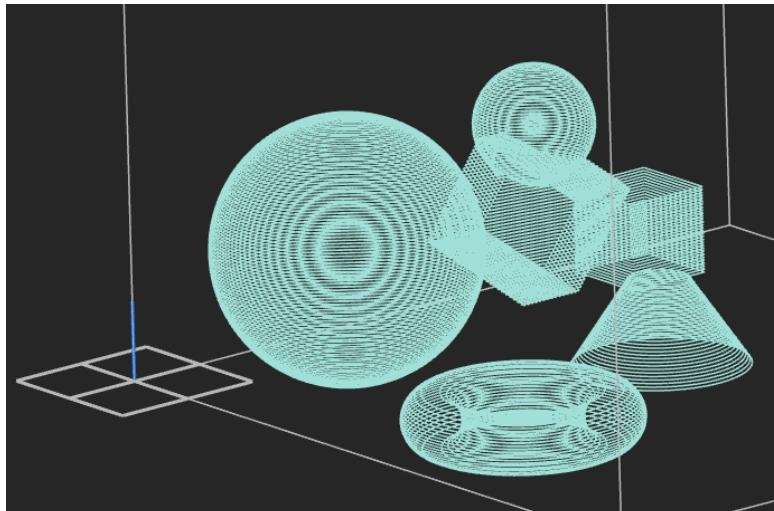
**Step 3:** Use the export **Slices to EOS** block and place the Part Slices variable into the slice stack input. Keep the supports unchecked and use the ASCII format.
