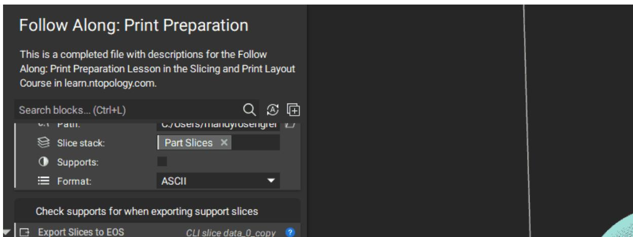
**Step 6:** For the body input of the CLI Slice Body by Tiers custom block, place the Min Sup. Orientations variable, located in the orienting parts section of the notebook. For the slice height, use 1mm, 7 for the slices per tier, and 1 for the slice feature size. For the tier number for export, we will use the **Sequence** block. If you are unfamiliar with the Sequence block, please visit our Intro to Automation course linked in the description.
