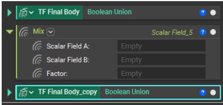
**Step 16:** Rename 'TF Final Body\_copy' to 'Mixed Final Body'. Make the Mix block a variable called 'Mix' and use it as input in the implicit body list within the 'Mixed Final Body' block.
