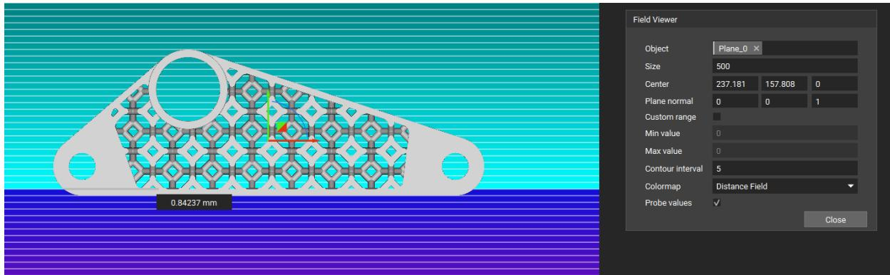
Notice the value of the field is zero where the plane is placed and increasingly positive in the direction of the normal the farther away from the plane.
