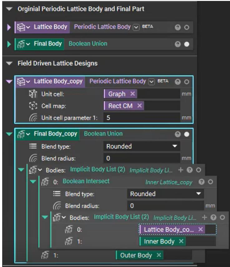
The following steps will create multiple different design variations for the latticed bracket by varying **Periodic Lattice** block's Unit cell parameter 1, which defines the lattice beam thickness.
