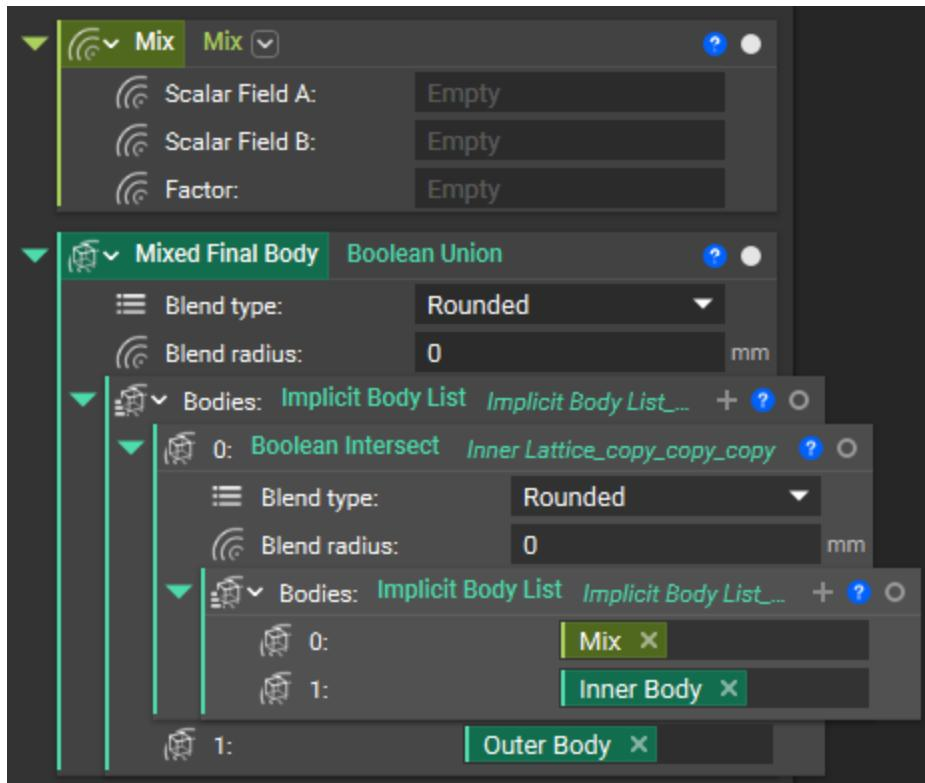
**Step 17:** For Scalar Field A input, use the implicit property of the 'TF Lattice Body'. For Scalar Field B, use the Inner Body implicit.
