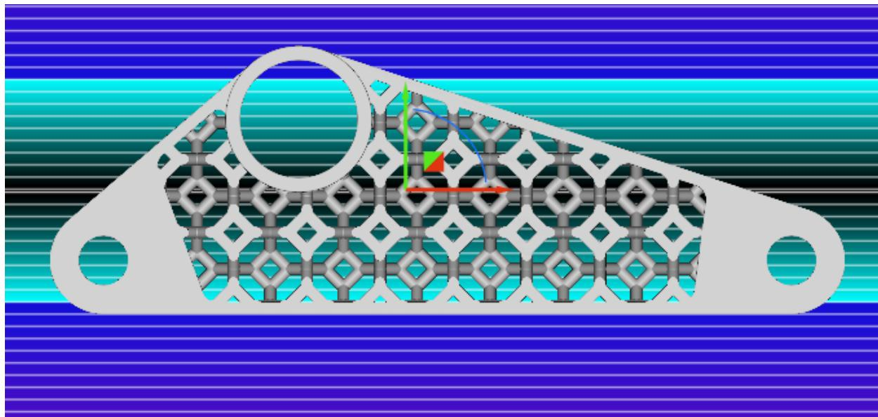
Notice the values of the field at the top and bottom of the lattice structure where the two planes are placed are 0 and both increasingly positive in their normal directions, reaching a maximum value at the midpoint between the two planes.
