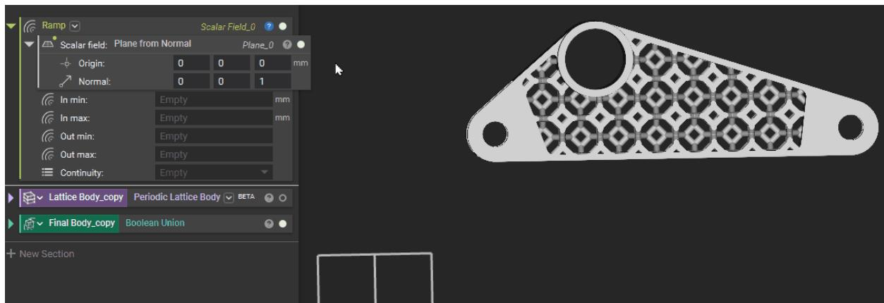
**Step 4:** Select the **Plane from Normal** Block and press 'F' on the keyboard to view its field with the visibility of the original 'Final Body' turned on. Move the field to where the Bracket is then adjust its size to 500, give a contour interval of 5, and check probe values.
