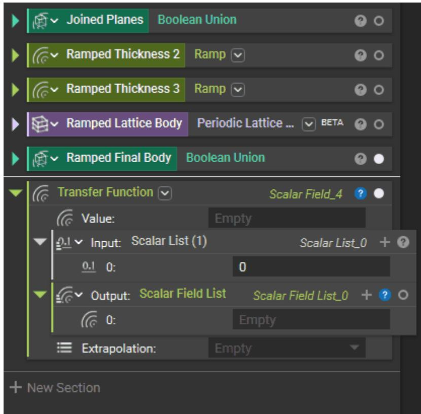
**Step 13:** Rename the two blocks to 'TF Lattice Body' and 'TF Final Body'. Make the Transfer Function block a variable called 'TF' and input it into Unit cell parameter 1. TF stands for Transfer Function.
