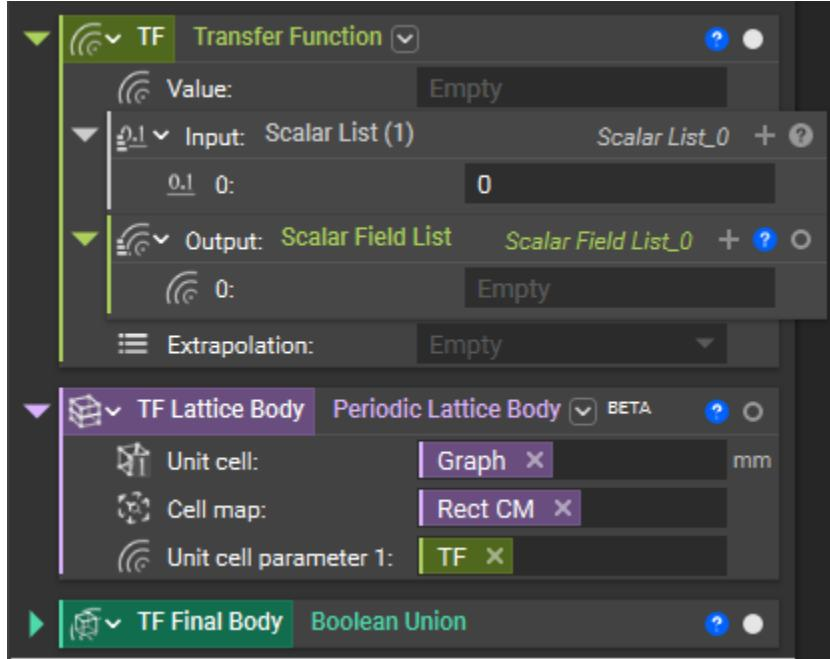
**Step 14:** In the value input of TF, use a **Plane from Normal** block with the same origin as 'Ramp Plane' and set the normal to [1,0,0]. View the field of this plane to probe input values at desired locations on the lattice structure and fill out the output thickness values. Make sure to include units. Choose clamped extrapolation.
