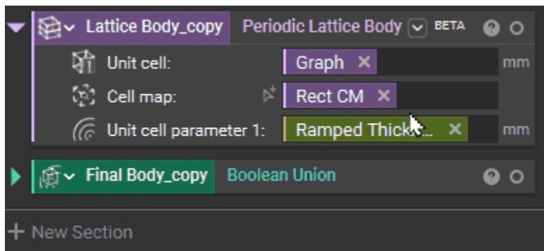
**Step 9:** Add a new **Ramp** block to the Notebook. For the Scalar Field, create 'Large Hole' Implicit body by converting the CAD surface into an implicit body and using **Thicken Body** block to add 1 mm thickness to the surface.
