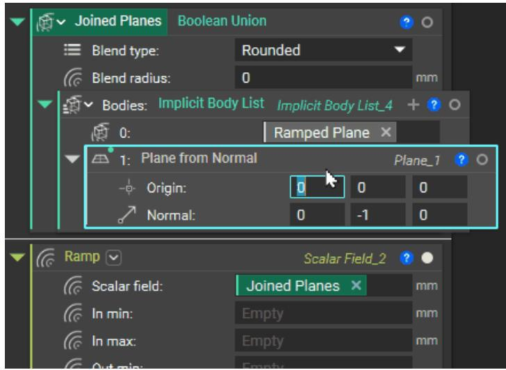
Turn off the visibility of the **Boolean Union** block and view its field with the original 'Final Body' turned on, using the same Field Viewer settings as in **Step 4** to probe for in min and in max values.
