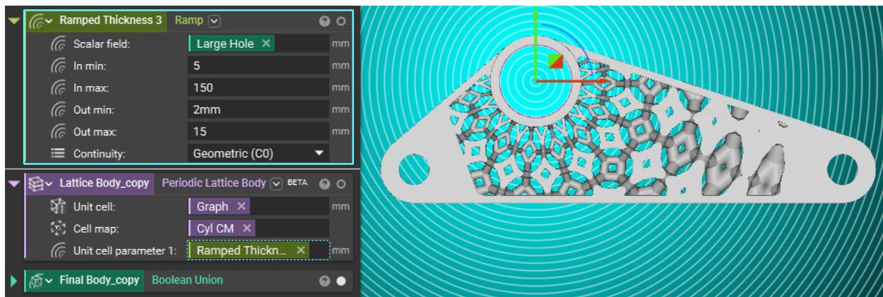
**Step 11:** Rename 'Lattice Body\_copy' and 'Final Body\_copy' to 'Ramped Lattice Body' and 'Ramped Final Body' respectively. Collapse all blocks.
